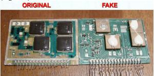
**Figure4** – Two "opened" electronic devices: on the left the original one, on the right the counterfeit one.
