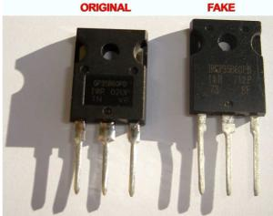
Figure5 – Two IGBTs IRGP35B60PD: the original one on the left, the conterfeit one on the right.
