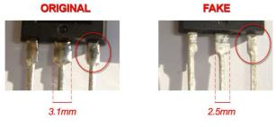
Figure7 - Detail of the legs of the two components
