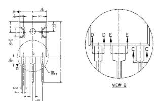
**Figure6** – Dimensioned drawing of the component (image taken from the original manufacturer's datasheet)
