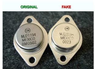
**Figure2** – Two power-transistors: on the left the original, on the right the counterfeit one.
